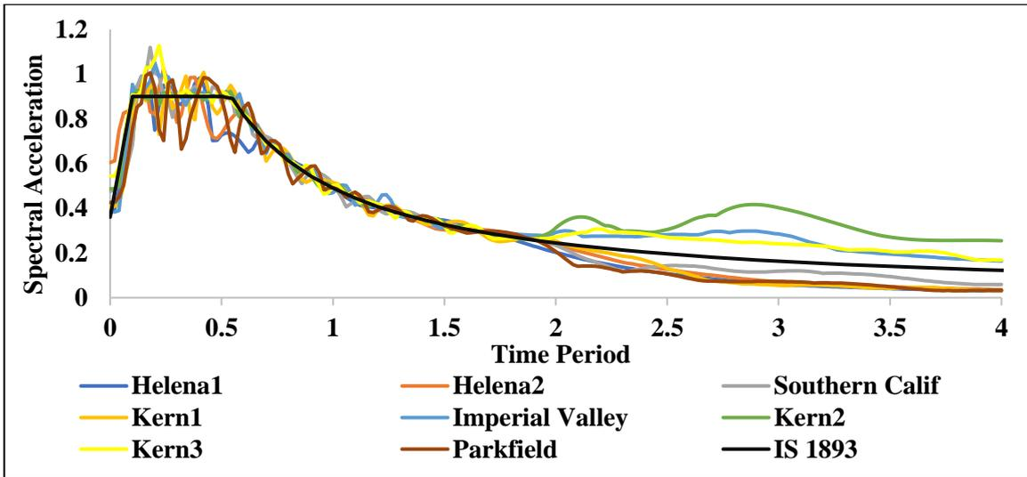
Figure 3: Response spectra of scaled ground motions
