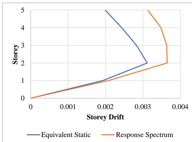
**Figure 2:** Average inter-storey drift plot for equivalent static and response spectrum analysis.
