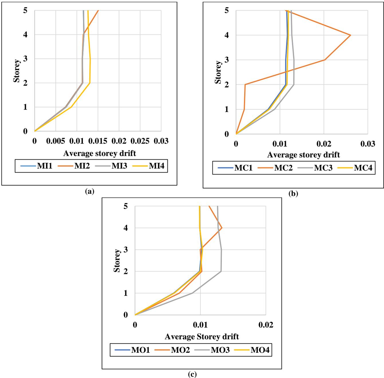
**Figure 5: Inter-storey drift for all ground motions (a) When walkway width is 2m (MI type), (b) When the walk way width is 3m (MC type) and (c) When the walk way width is 4m (MO type)**
