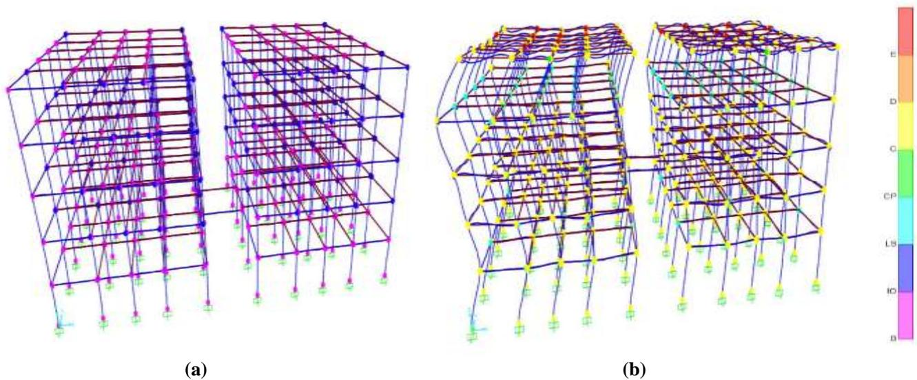
**Figure 6 Plastic hinge formation (a) For MO1 model for Parkfield ground motion
