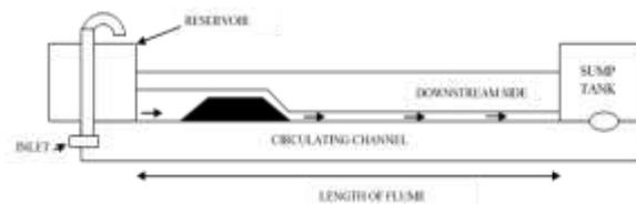
Fig. 3: Line diagram of flume
