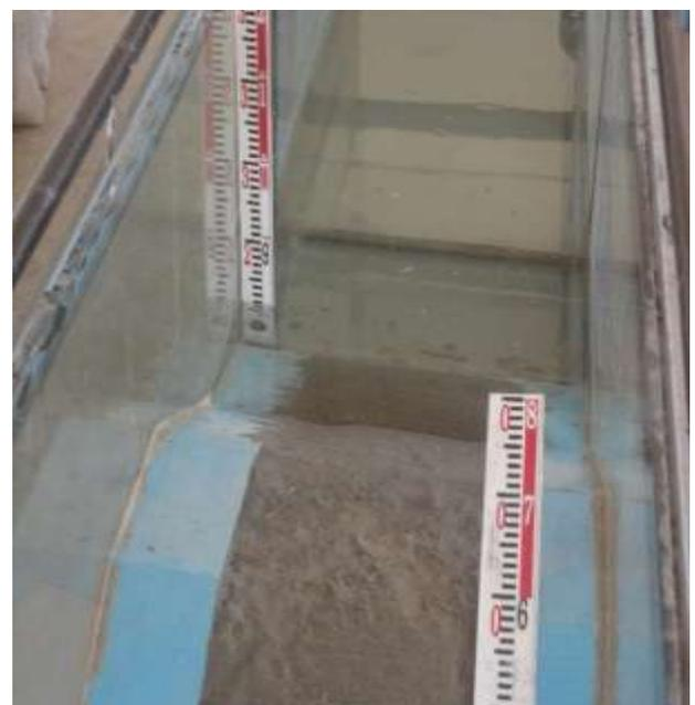
Fig. 4b: Saturation of embankment
