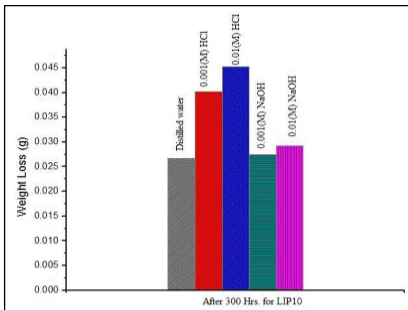
Figure 3: Bar Diagram of Wt. loss in different medium after 300 hours for LIP10 glass.
