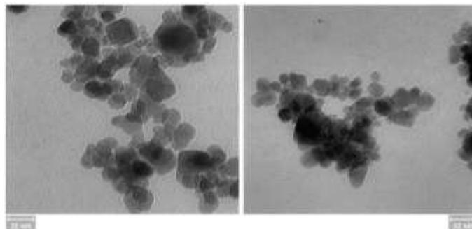
**Fig. 1: TEM images of  $\text{Fe}_3\text{O}_4$  and  $\text{Fe}_3\text{O}_4$ -PEG magnetic NP**
