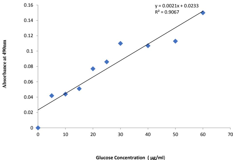
Figure 2: Standard curve of glucose
