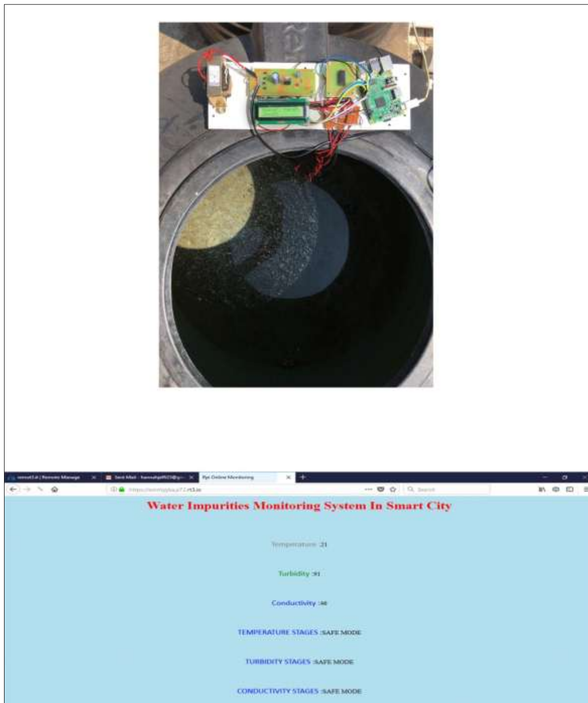
Figure 8: Practical Application in Drinking Water
