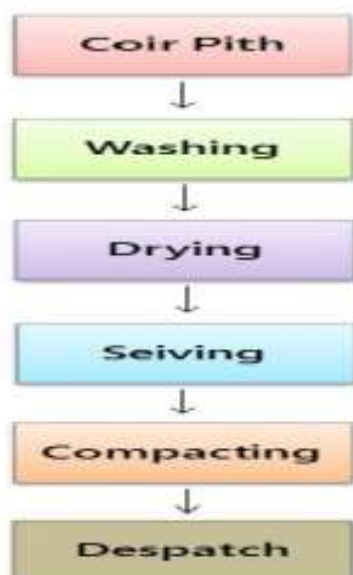
Fig. 4: Process flow of coir pith block manufacturing
