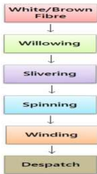
Fig. 3: Process flow of coir yarn spinning
