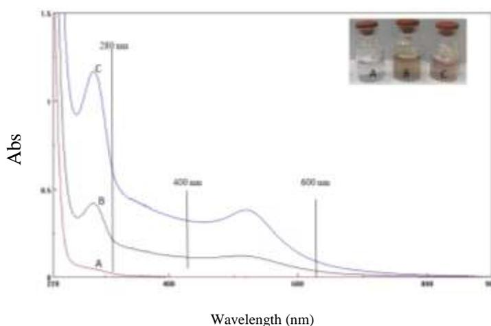
Figure 8: AuNP-PAMAM G3.0 stability at (A) pH 2, (B) 7 and (C) 9 in saline solution after being stored in an incubator at 37°C for 7 days
