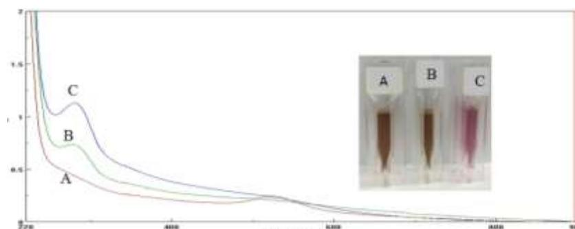
Figure 3: Overlay of gold nanoparticles (AuNP) encapsulation in polyamide amine generation 3.0 (AuNP-PAMAM G3) UV-Vis spectrum at (A) pH 2, (B) 7 and (C) 9
