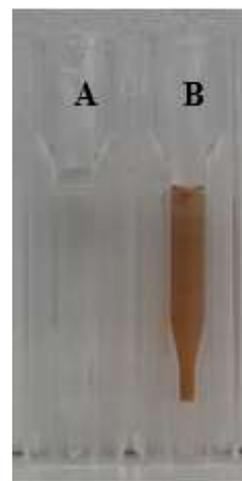
**Figure 1: A. Mixed solution of HAuCl<sub>4</sub> and PAMAM G3.0, B. Mixed solution of HAuCl<sub>4</sub> and PAMAM G3 after adding sodium borohydride (NaBH<sub>4</sub>)**
