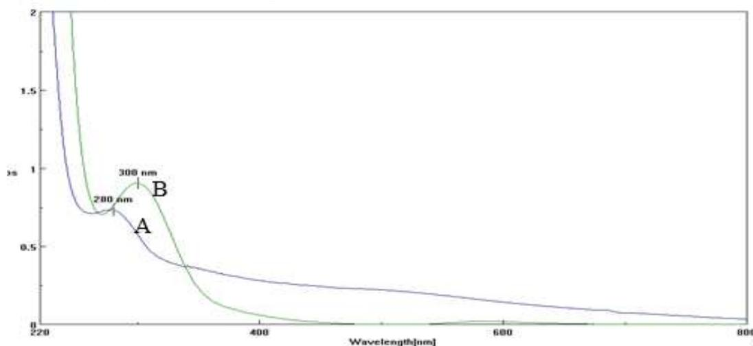
Figure 2: Overlay of the UV-Vis Spectrum: A. Gold nanoparticles (AuNP) encapsulation in polyamide amine (PAMAM) dendrimer generation 3.0 [AuNP-PAMAM G3] and B.  $\text{HAuCl}_4$  solution
