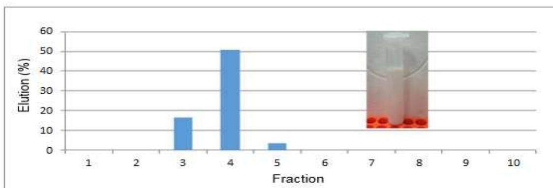
Figure 6: Efficiency of <sup>198</sup>AuNP-PAMAM G3.0 pH 7 after passed through Sephadex PD-10 column
