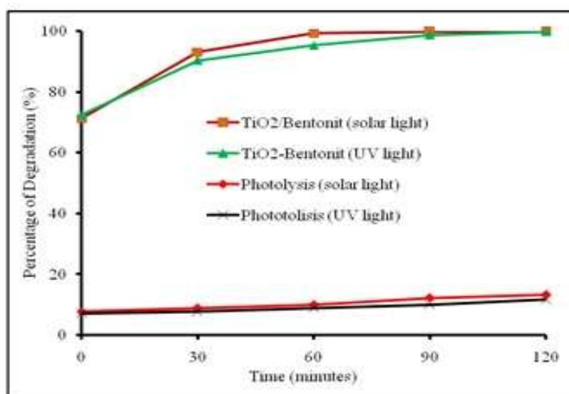
Figure 7: Photocatalytic and photolysis degradation of NBB. Initial dye concentration is 5 mg/L, initial pH solution is 3 and photocatalyst dosage is 0.4 g.
