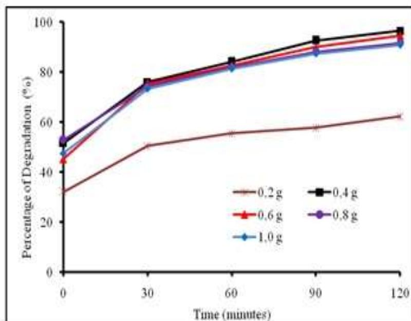
Figure 5: Photocatalytic degradation of NBB under UV light irradiation at various photocatalysts dosage. Initial dye concentration is 15 mg/L, initial pH solution is 3.
