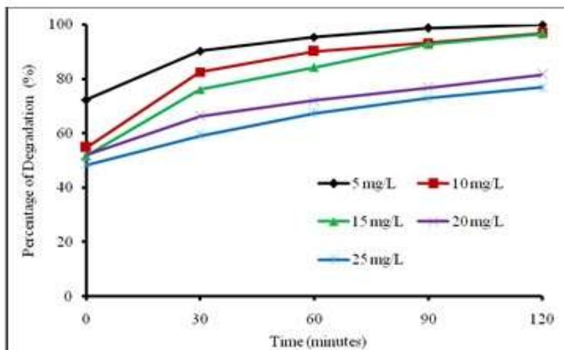
Figure 6: Photocatalytic degradation of NBB under UV light irradiation at various initial dye concentration. Initial pH solution is 3 and photocatalyst dosage is 0.4 g.
