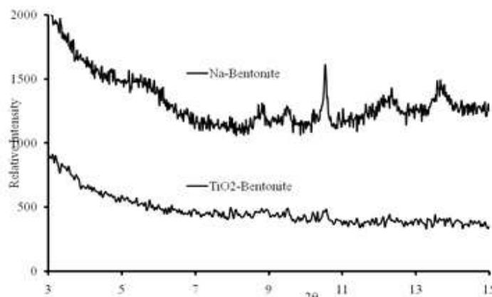
Figure 2: XRD pattern of the natural bentonite and TiO<sub>2</sub>/bentonite composite
