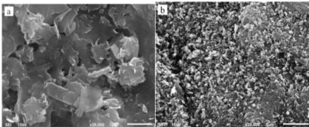
Figure 3: SEM image of a. Natural bentonite and b. TiO<sub>2</sub>/bentonite composite
