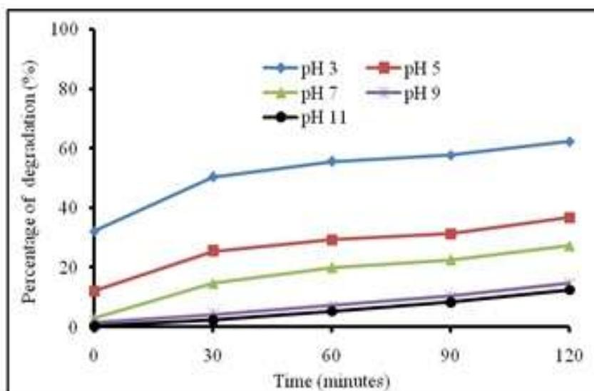
Figure 4: Photocatalytic degradation of NBB under UV light irradiation at various initial pH solutions. Initial dye concentration is 15 mg/L, photocatalyst dosage is 0.2 g.
